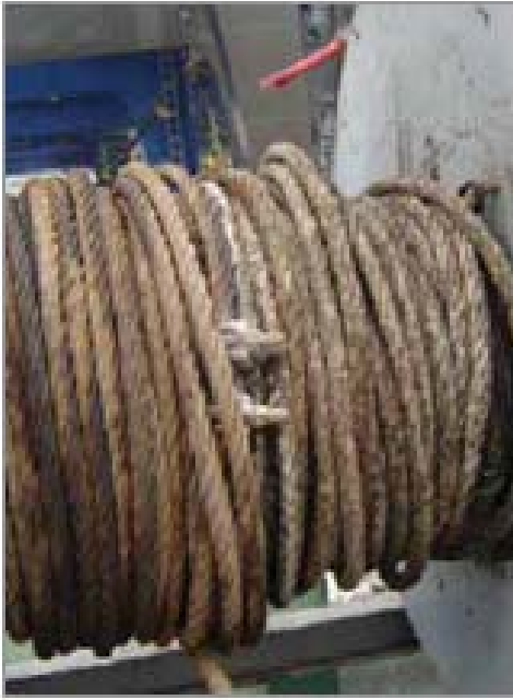
Badly spooled corroded mooring wire
