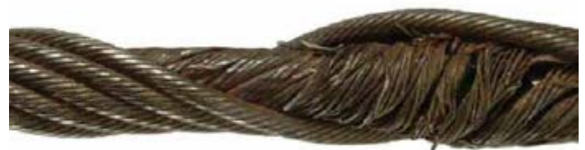
Multi-strand rope that has parted due to internal corrosion
