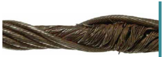
Multi-strand rope that has parted due to internal corrosion
