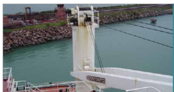
Badly spooled corroded mooring wire
