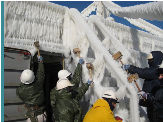
Crew removing ice buildup from a vessels structure
