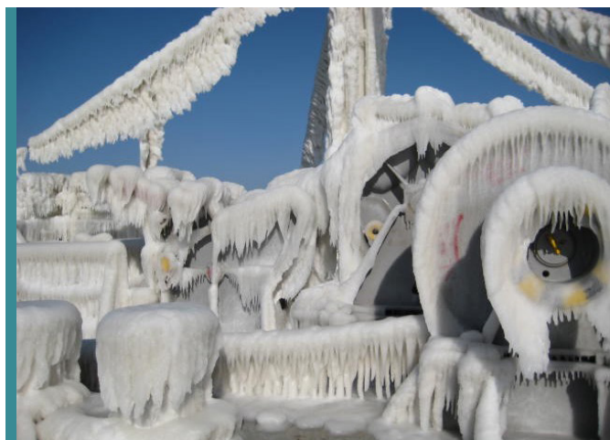
A vessels foremast with ice accretion
