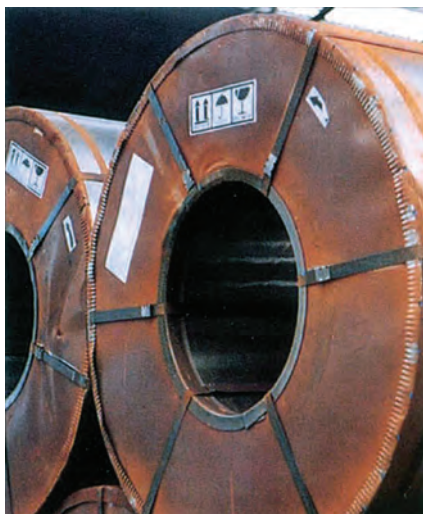
Fig. 2. Wrapped coils. Surface-condition clause: packing rust stained
