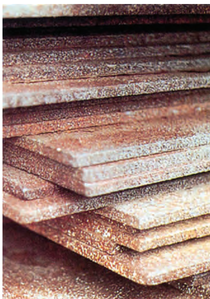
Fig. 10. Plates. Surface-condition clause: rust with pitting
