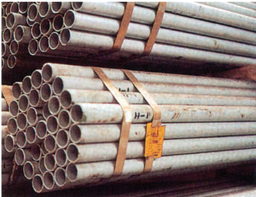
Fig. 15. Galvanised pipes bundles showing no evidence of having been subjected to a passivation process. Surface-condition clause: galvanising dull
