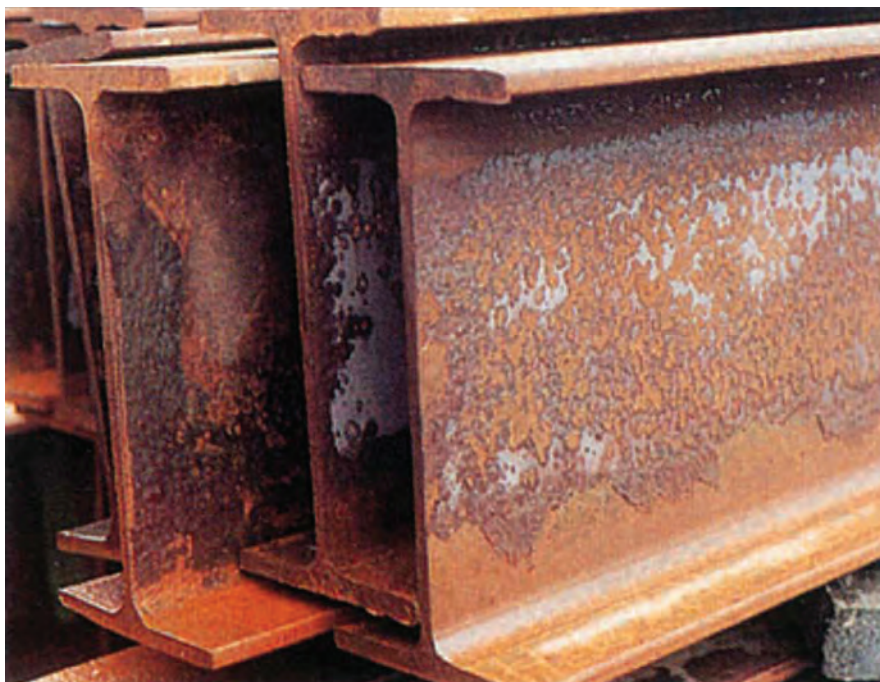
Fig. 16. Beams with flaking mill scale on webs. Surface-condition clause: rust stained, rust spots apparent
