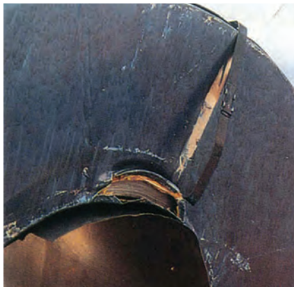
Fig. 18. Wrapped coil damaged by forklift. Mechanical-damage clause: packing torn open in one place at inner circumference. Visible cargo is scored. Affects 15 windings
