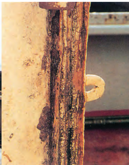
Fig. 29. Mast house door leading to a cargo hold internal escape hatch. Closer examination reveals that the door's sealing rubber has been painted over and is hardened, excessively compressed and perished leaving the cargo vulnerable
