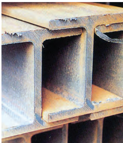
Fig. 6. Beams with some mill scale still intact but rust encroaching on flanges and webs. Note correct nesting position. Surface-condition clause: rust stained
