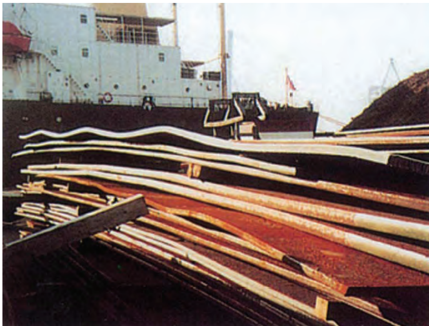
Fig. 22. Plates. Mechanical-damage clause (top plate in stack): edges waved along entire length
