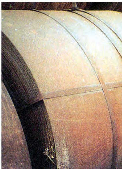
Fig. 8. Hot-rolled steel coils. Surface-condition clause: rusty
