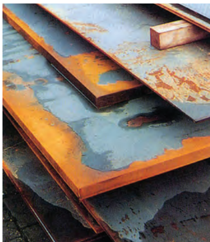
Fig. 5. Plates with most mill scale intact, but handling has also fragmented mill scale from edges. Surface-condition clause: partly rust stained, wet before shipment
