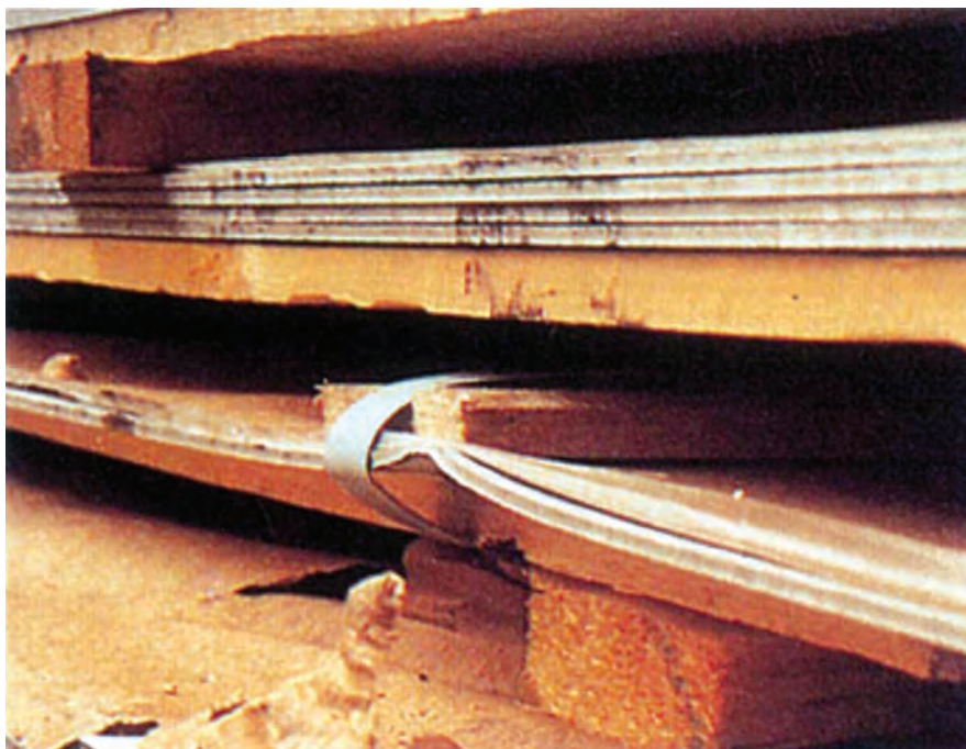
Fig. 25. (above) Bundle of stainless steel plates. Mechanical-damage clause: edges dented at centre where handling gear marked. Affects two plates
