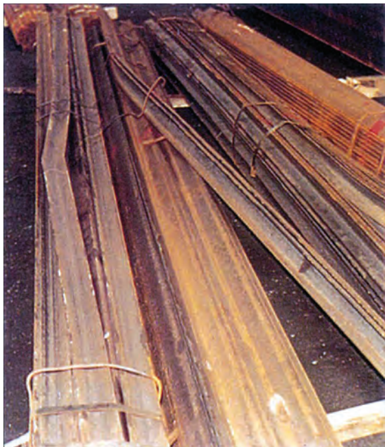
Fig. 23. Bundles of light scantling pieces. Mechanical-damage clause (second bundle from left): bundle pieces bent along entire length. Affects two pieces. Strapped insufficiently, one strap broken, three missing
