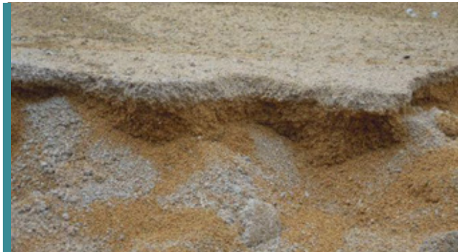
Caking from self-heating.
