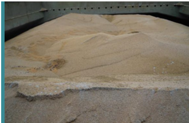
Discolouration from self-heating.
