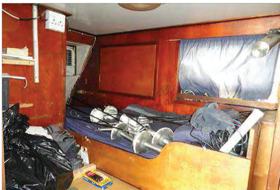
Answers: 1. Electrical socket wiring insulation poorly repaired with electrical tape 2. Using cabin to store equipment and parts 3. Storage of combustibles 4. Obstructed movement within cabin 5. A prize for any others you can find email - loss.prevention@nepia.com
