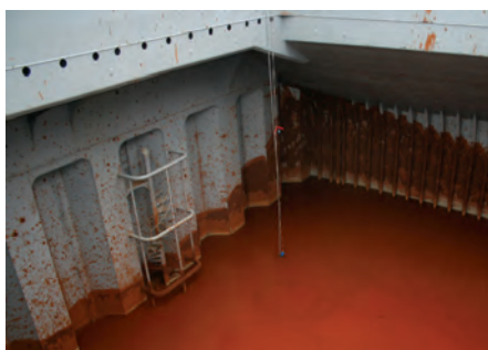
Nickel ore with excessive moisture content. Source: Ken Grant.
