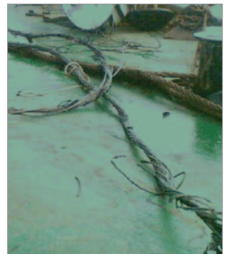
A submarine cable damaged by an anchor
