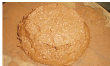
Sample cone after testing with 20 mm expansion at base
