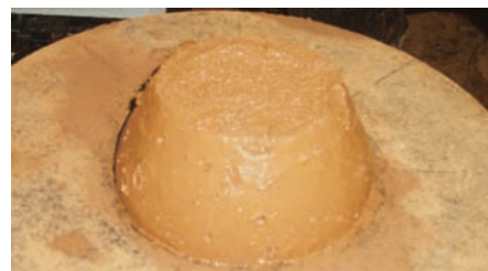
Change in shape of sample cone after testing, corresponding to a 6.5 mm cone expansion
