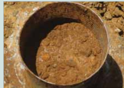
Appearance of moisture on surface of nickel ore following a can test
