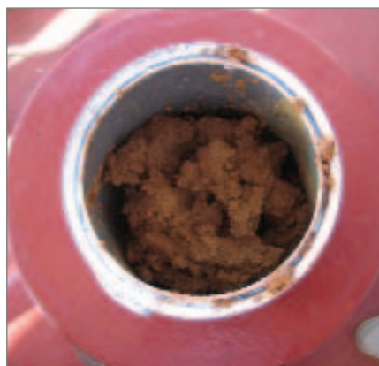
Figure 2. Liquid state – after a 'can' test – no friction between particles
