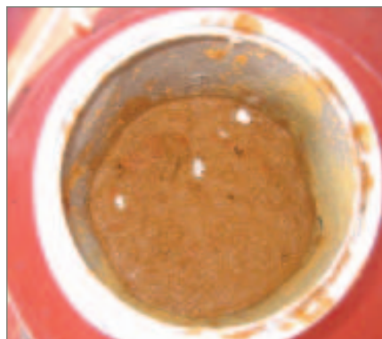
Figure 2. Liquid state – after a 'can' test – no friction between particles
