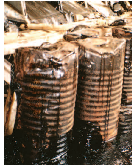
Leaking bitumen drums
