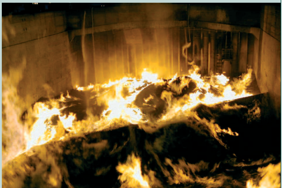
DRI cargo on fire
