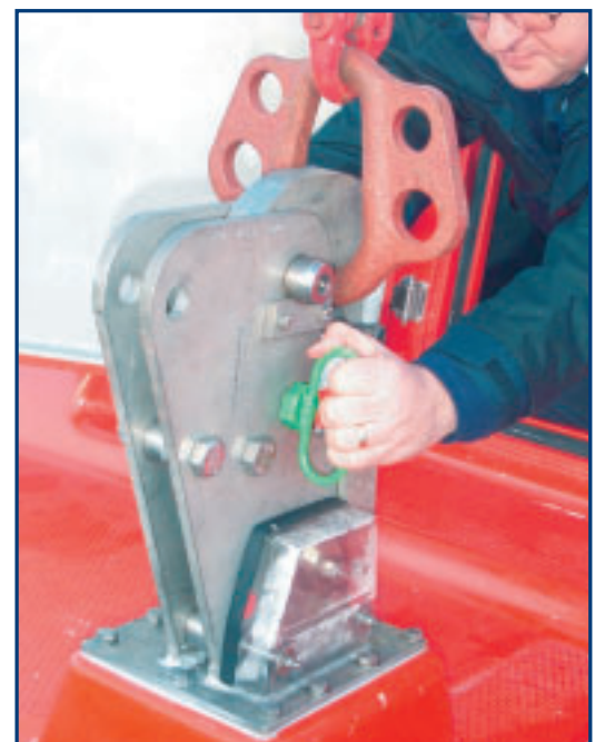
The new on-load release hook with locking pin.
