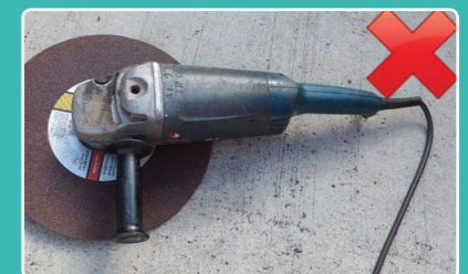
Worn down disc should not be used to carry out a task.
