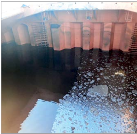
Flooded cargo hold
