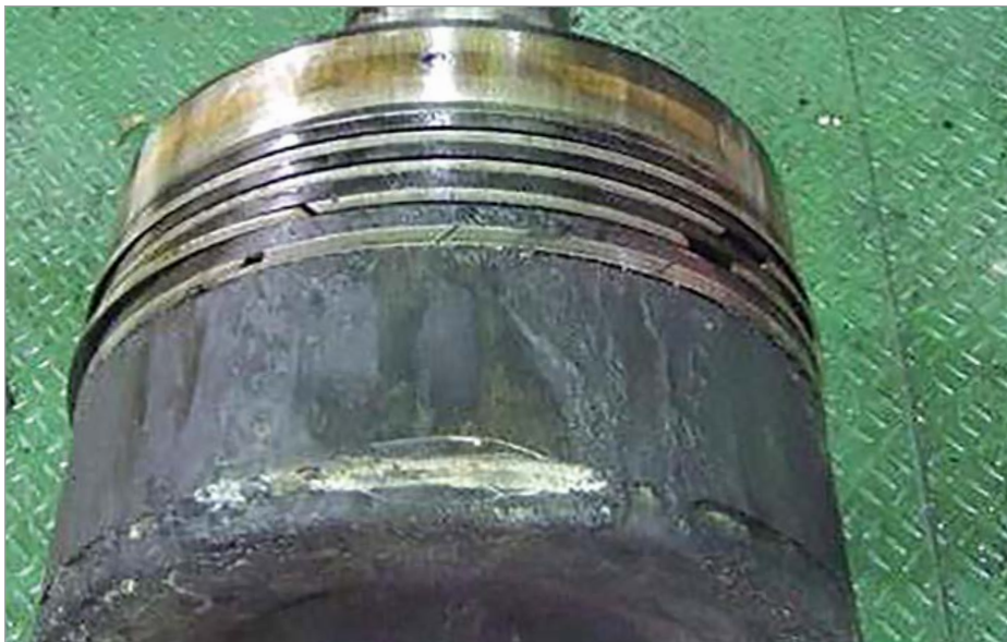
Broken piston rings caused by cat fines. Image courtesy of Braemar Salvage Association
