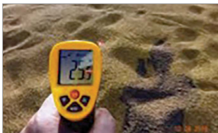
Cargo temperature on loading should not change much during the voyage. An increase in cargo temperature is an indication of self-heating.
