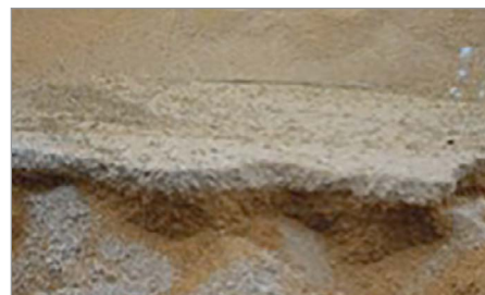
Caking from self-heating.
