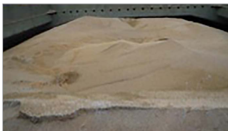
Discolouration from self-heating.
