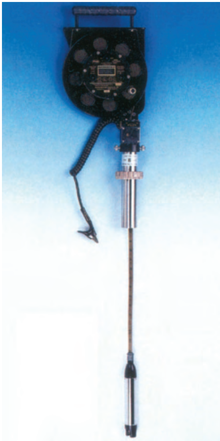
Fig. 9. Typical portable gauging device for closed-loading systems. This device measures the ullage, temperature and oil/water interface
