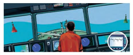
Large waves and swell can act to reduce the under-keel clearance of a vessel by actually reducing the available depth of water and/or by causing a vessel to roll heavily. These are factors that need to be taken into account when passing through constrained waters. Ask yourself whether or not the sea state is going to reduce the available depth of water to an extent that it might put a vessel at risk. If it might then perhaps the evolution should be delayed until the weather abates.
