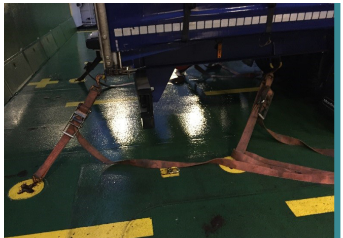
Fig 2: Lashing should be suitable for vehicle type and weight
