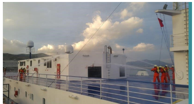
Fig 14: Fire drill - boundary cooling
