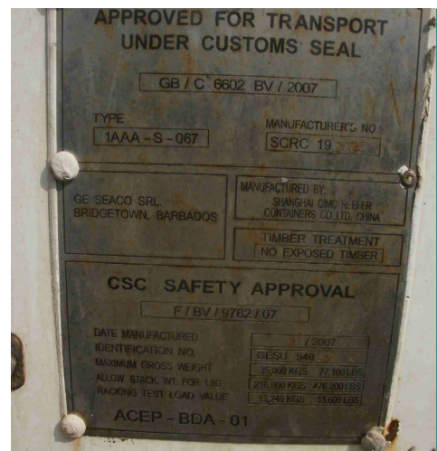
Figure 7: Container CSC Plate
