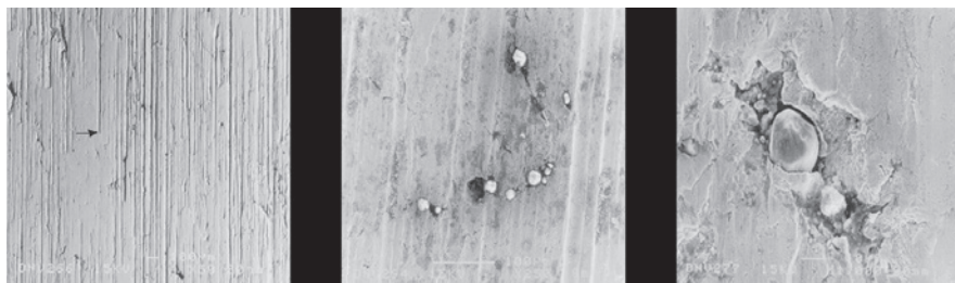
Fig. 4. Microscopic image of cat fines damage to piston ring of main engine (VPS)
