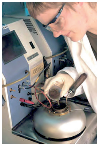
Fig. 3. The flashpoint of a fuel is an important characteristic and should be accurately measured in a laboratory (VPS)
