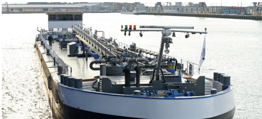
Fig. 6. Typical bunker supply vessel – often referred to as a ‘bunker barge’ (VPS)
