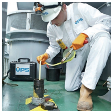
Fig. 11. Surveyor carrying out tank sounding to determine quantity (VPS)
