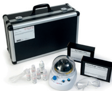
Fig. 20. On-board testing kit for cat fines (Parker Kittiwake)
