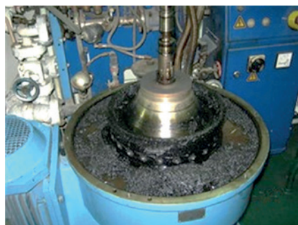
Fig. 19. A simple on-board stability / compatibility test can avoid choked purifiers (Braemar Salvage Association)
