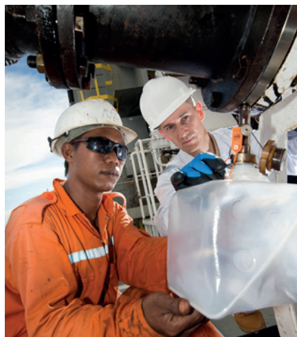
Fig. 16. Fitting a sampling container to the bunker manifold (VPS)
