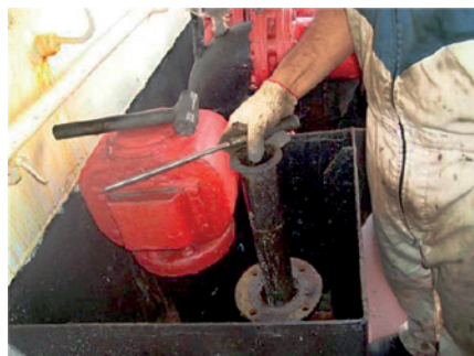
Fig. 15. Removing an insert within a sounding pipe (Maritech Commercial Inc.)
