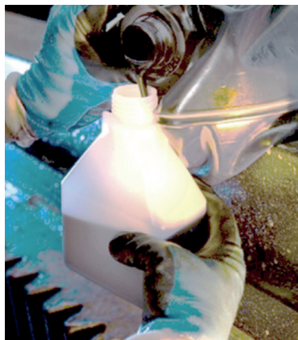
Fig 17. Filling sample bottles for dispatch to laboratory for testing (VPS)
