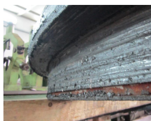
Slewing bearing inner flange with circumferential deep scoring
