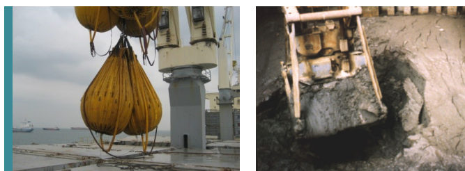
Example of a static load test using water bags and potential dynamic loading situation from a wet bulk cargo
