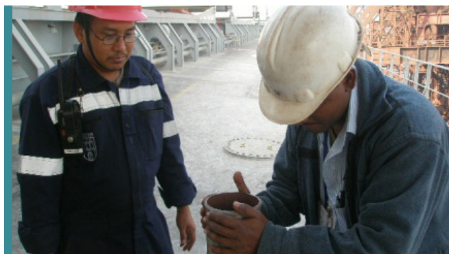
Figure 4: Can test of cargo
