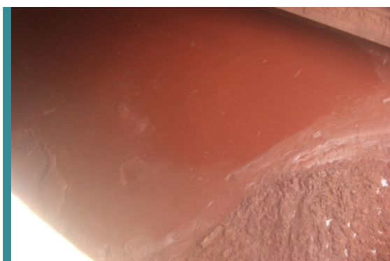
Figure 6: Liquefaction Iron Ore Fines in a Cargo Hold
