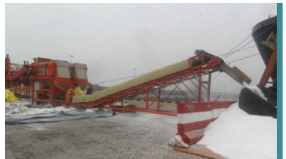
Conveyor dumping cargo at loading berth
