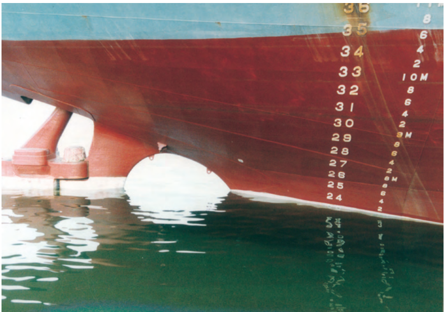
Figure 12. (Below) Misplacement of marks aft (Paul Coombs)
