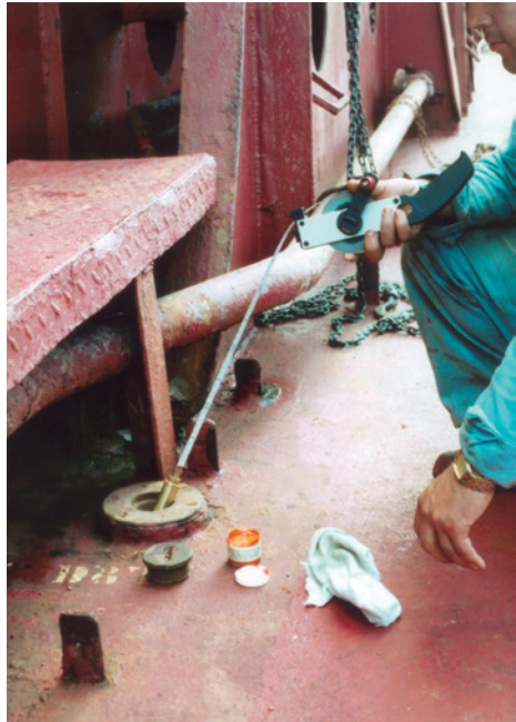
Figure 3. Using a sounding tape
