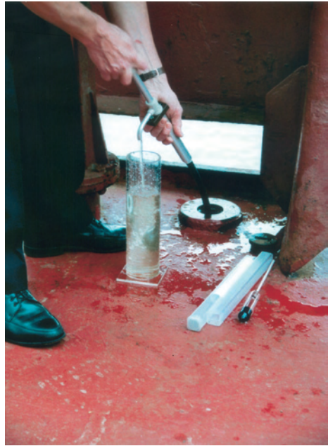
Figure 4. Taking a ballast sample
