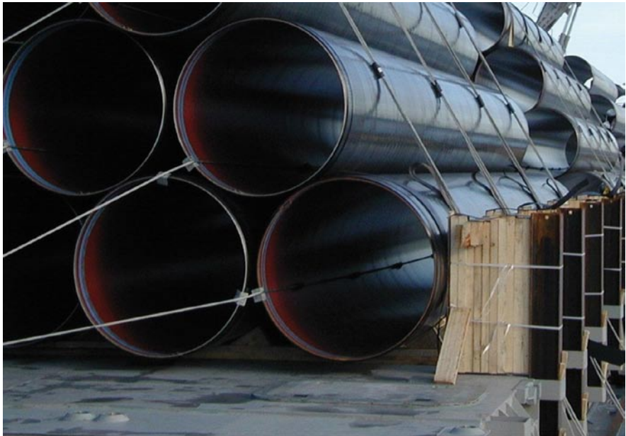
Fig. 8. This stowage incorrectly combines securing alternatives two and three, but the horizontal halfloop lashings are effectively redundant as the stanchions prevent them stretching sufficiently to carry any appreciable load
