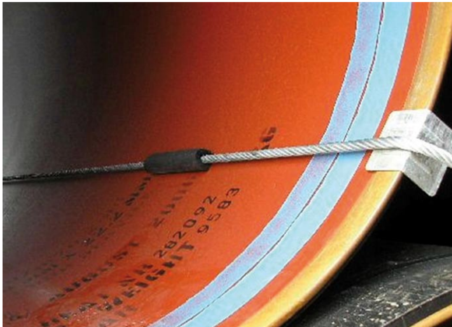
Fig. 11. Pipe edge protectors and rubber-hose sheaths should be used with horizontal half-loop lashings
