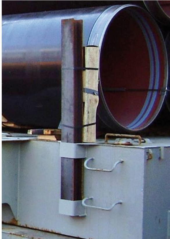
Fig. 12. Stanchion concept one – short lengths of steel I-beams are inserted into steel lugs welded to the hatch-cover sides or coamings
