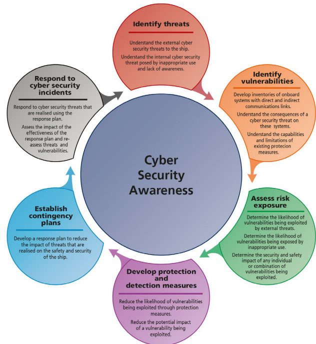
Cyber security awareness - Closing the loop. From Guidelines on Cyber Security Onboard Ships Published by BIMCO
