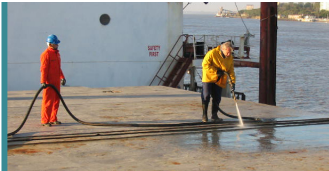
Hose testing of cargo hatch lids.
