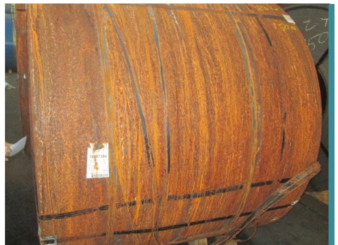
A rusted steel coil pre-shipment
