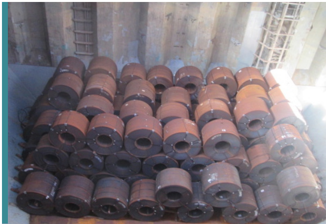
Rusted cargo of coils in a ships hold
