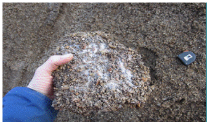
Example of a seed cake cargo where there has been microbiological activity resulting in mould growth and self-heating
