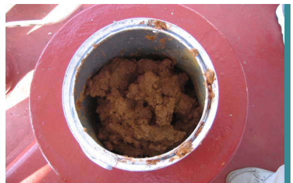
Figure 1 - Solid state - before a 'can' test - particles held together by friction
