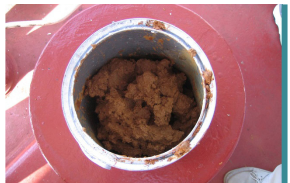
Figure 2 - Liquid state - after a 'can' test - no friction between particles
