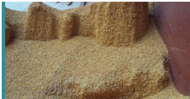
Heat damaged grain – stowed next to engine room bulkhead
