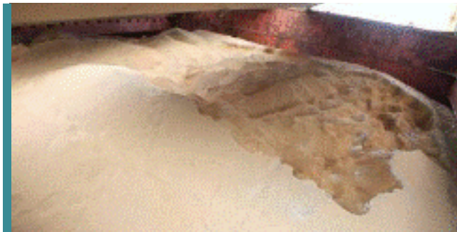
Grain cargo - wet damage from leaking hatch cover
