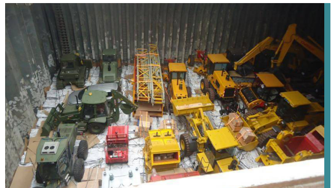
Example of poor loading practices with vehicles loaded over jumbo bags
