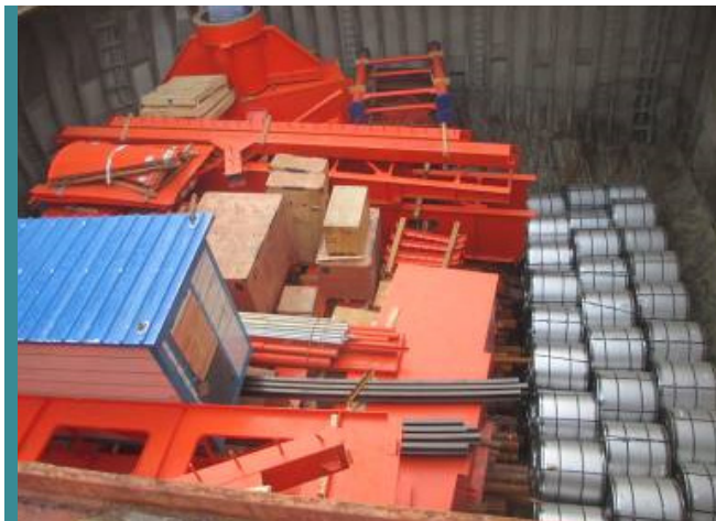
A typical break bulk load which may create problems when lashing
