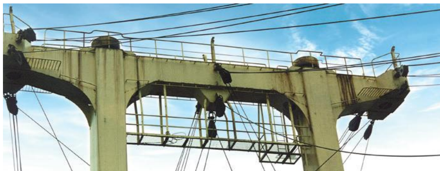
Fig. 15. Ventilator inlets can be positioned on top of king posts or masts
