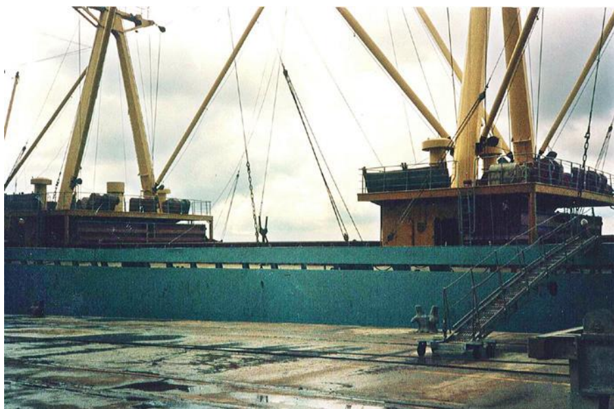
Fig. 16. Mechanical ventilation systems often have ventilators on mast houses which contain the fans
