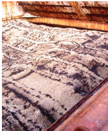
Fig. 2. Surfaces of cargoes can be heavily wetted if no ventilation is applied, resulting in a claim against the shipowner
