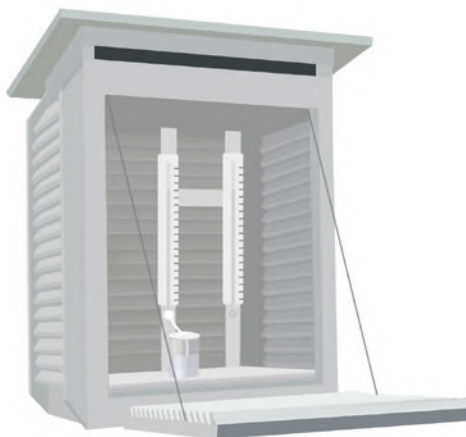
Fig. 6. Stevenson screen, normally located on a ship's bridge wing, contains wet-bulb and dry-bulb thermometers and is used to measure the dew point of the outside air
