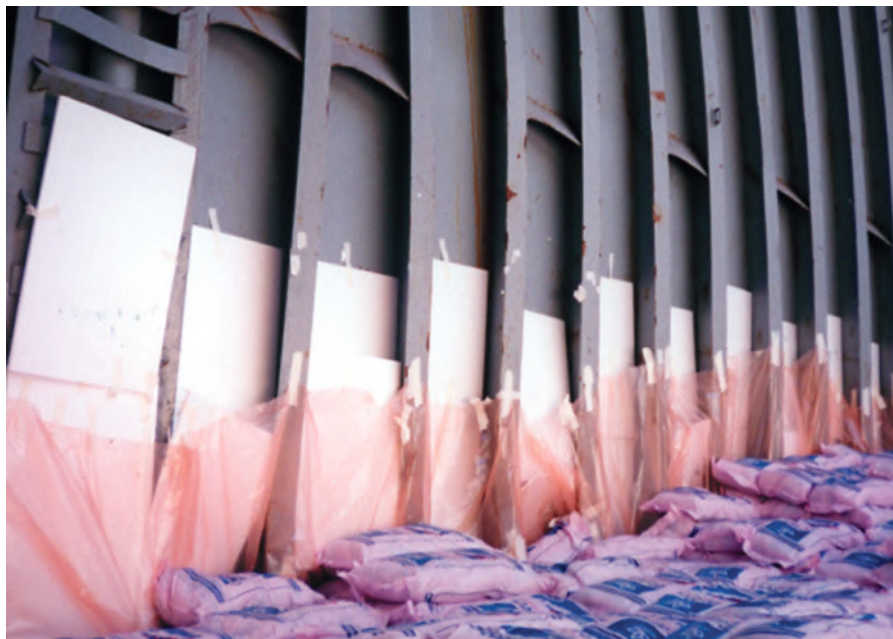
Fig. 20. Dunnage of foam-polystyrene sheets overlain by plastic sheeting (photo courtesy of Allied Maritime Inc.)
