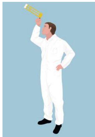
Fig. 7. Aspirated or 'whirling' psychrometer also contains wet-bulb and dry-bulb thermometers and is used to measure the dew point of the air in the hold
