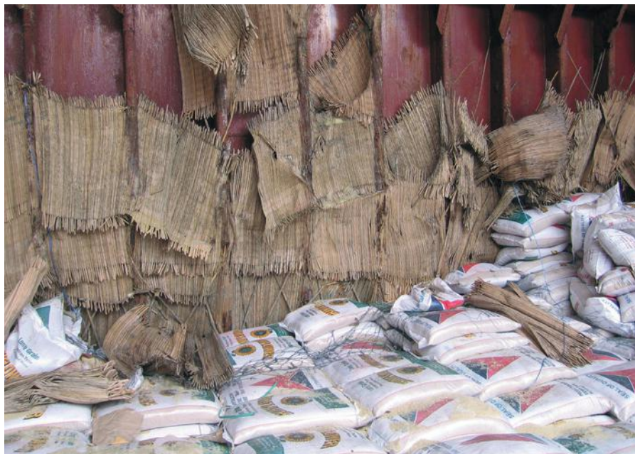
Fig. 19. Bamboo dunnage mats are often used with bagged rice cargoes. But unless they are kept clear of frames by dunnage planks or poles, they provide little protection against condensation
