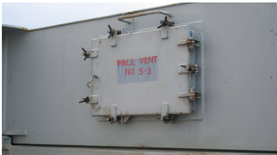
Fig. 14. Ventilators can be mounted on the side of hatch covers as well as on hatch coamings
