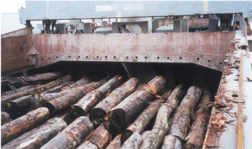
Fig. 16. Logs stowed under-deck
