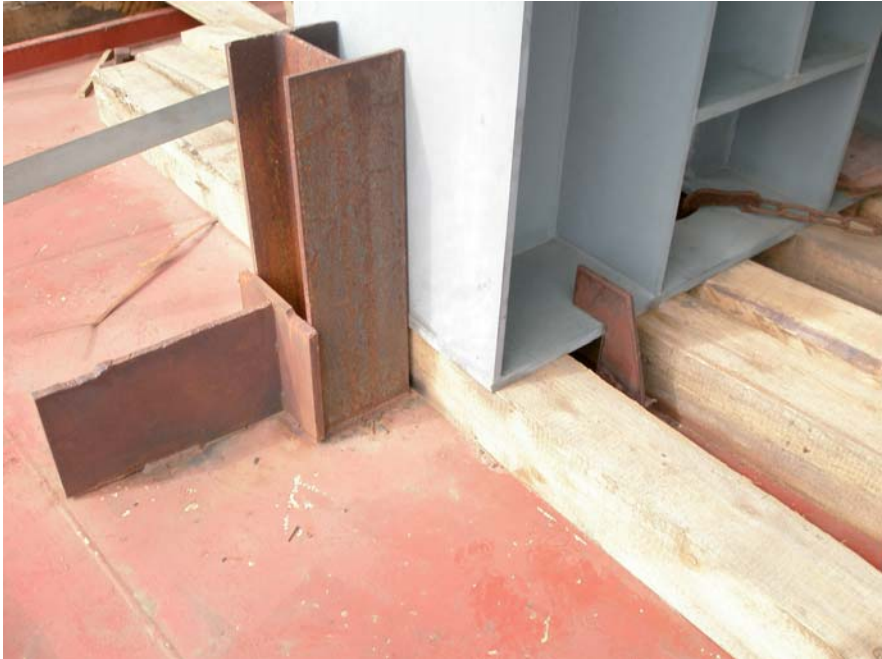
Fig. 12. Sea fastenings (Graig Ship Management Ltd)
