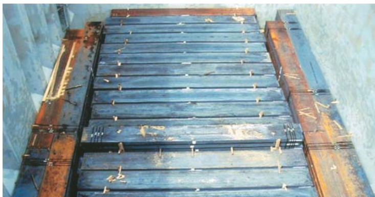
Fig. 10. California block stow
