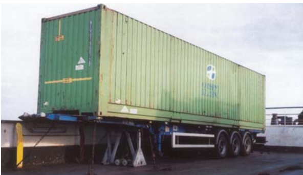
Fig. 13. Ro-ro container trailer secured on trestle
