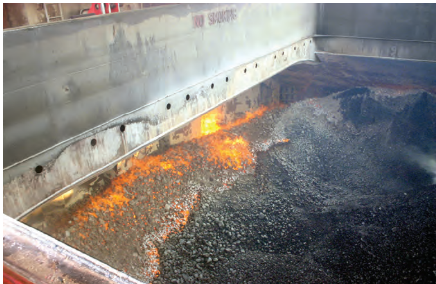
Fig. 33. Coal on fire in a ship's hold
