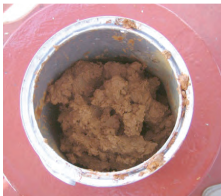
Fig. 26. Nickel ore in solid state before a can test – particles are held together by their friction
