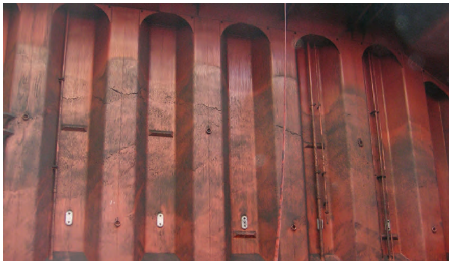
Fig. 9. An end bulkhead which displays black residues after the carriage of a coal cargo
