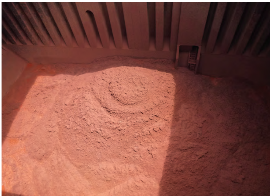
Fig. 28. A stowage of iron ore which has a high moisture content – wave markings can be seen in the pile caused by cargo dropped onto the pile from a height
