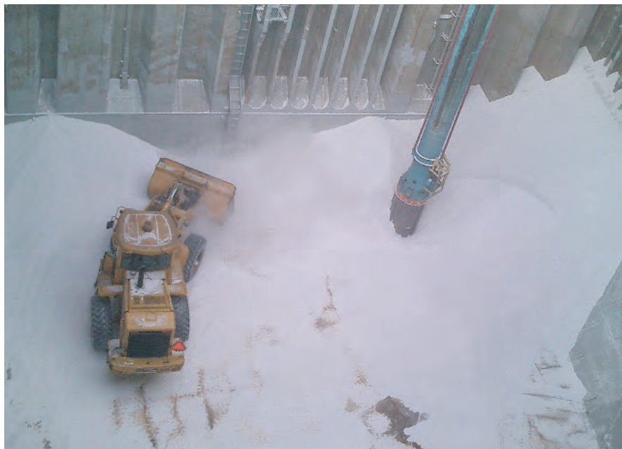
Fig. 40. Unloading salt by pneumatic suction pipe and with a front-end loader to trim the cargo to the pipe. Note the discoloured salt on the tank top plating
