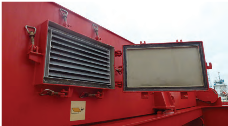
Fig. 6. Hatch-end ventilators must also be tested for weathertightness
