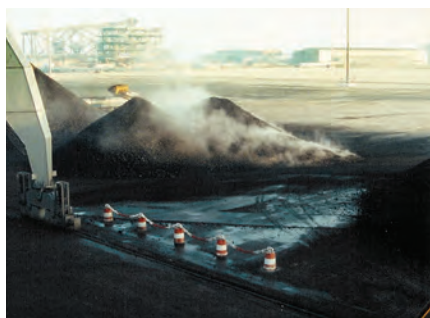
Fig. 32. Steam rising from coal in an on-shore stockpile which is wet from rainfall and heating up
