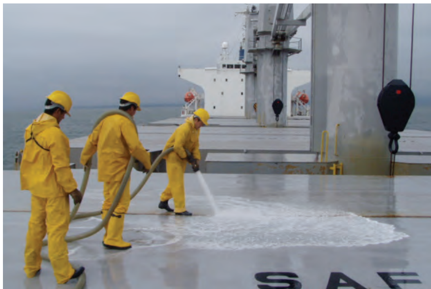
Fig. 3. Hose-testing of hatch covers
