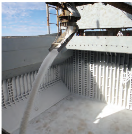
Fig. 39. Loading salt by conveyor and a spout with a directional head
