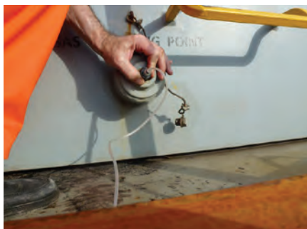
Fig. 34. A sampling port in the side of a hatch cover with the gas sampling tube inserted
