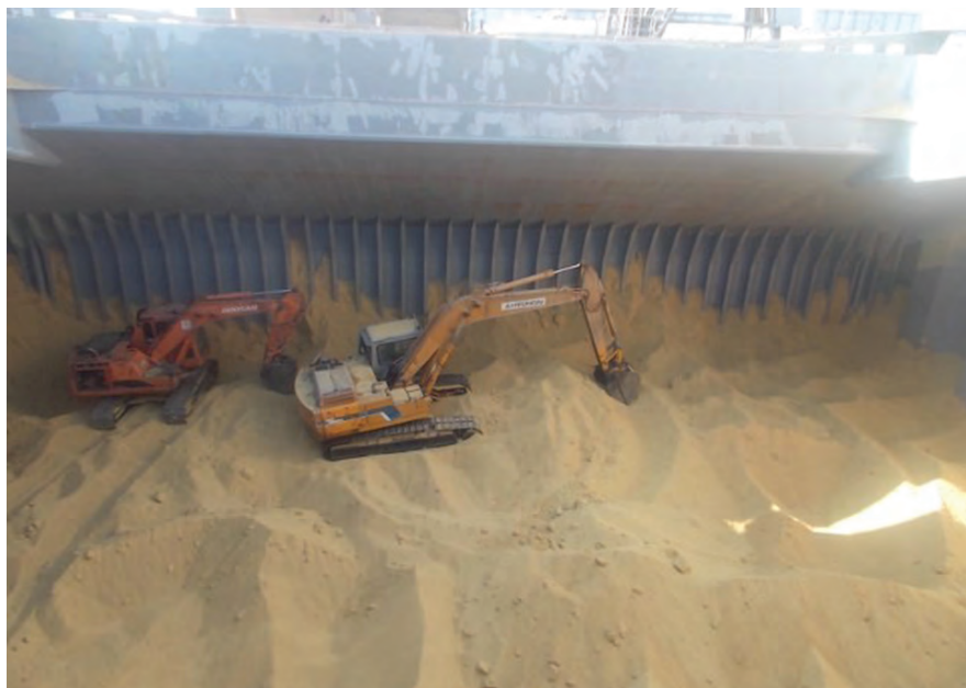
Fig. 41. Seed cake cargo being trimmed out from under the wing by back-hoes during unloading
