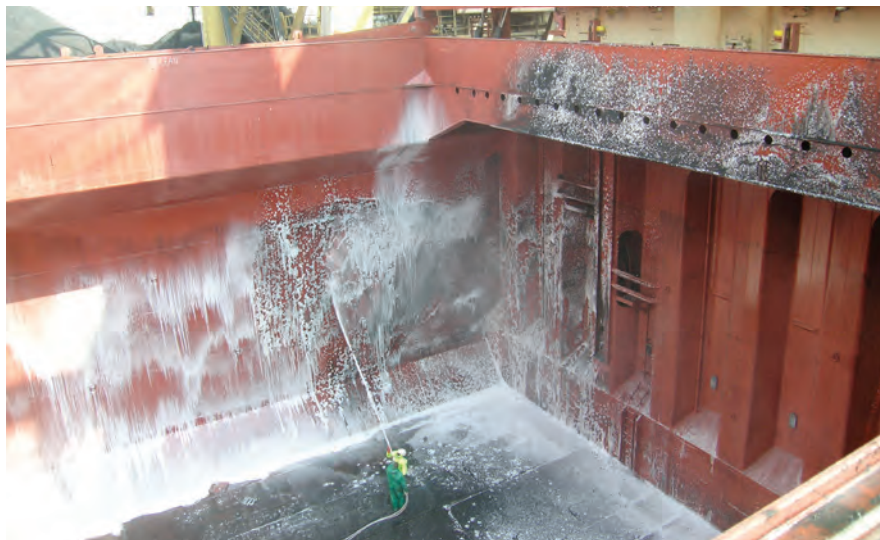
Fig. 14. A water cannon in use with a chemical cleaning product to clean the hold after a petcoke cargo
