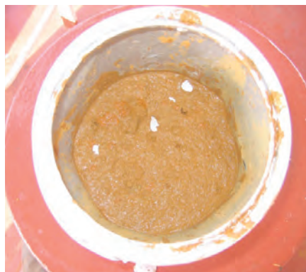
Fig. 27. Nickel ore in liquid state after a can test – no friction between the particles
