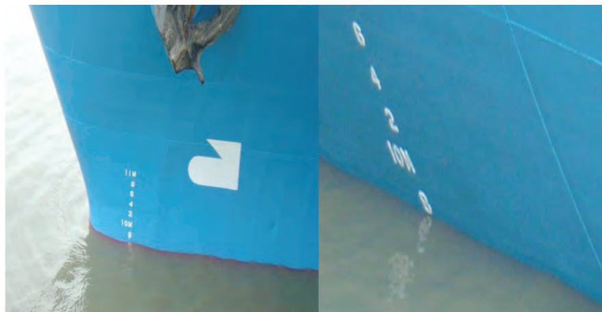
Fig. 20. Forward and aft draught marks
