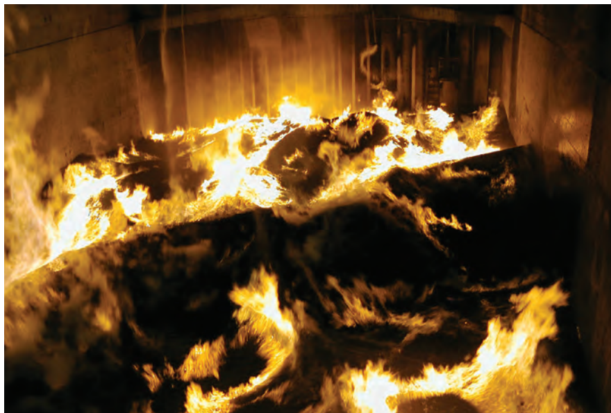
Fig. 37. DRI on fire in a ship's hold
