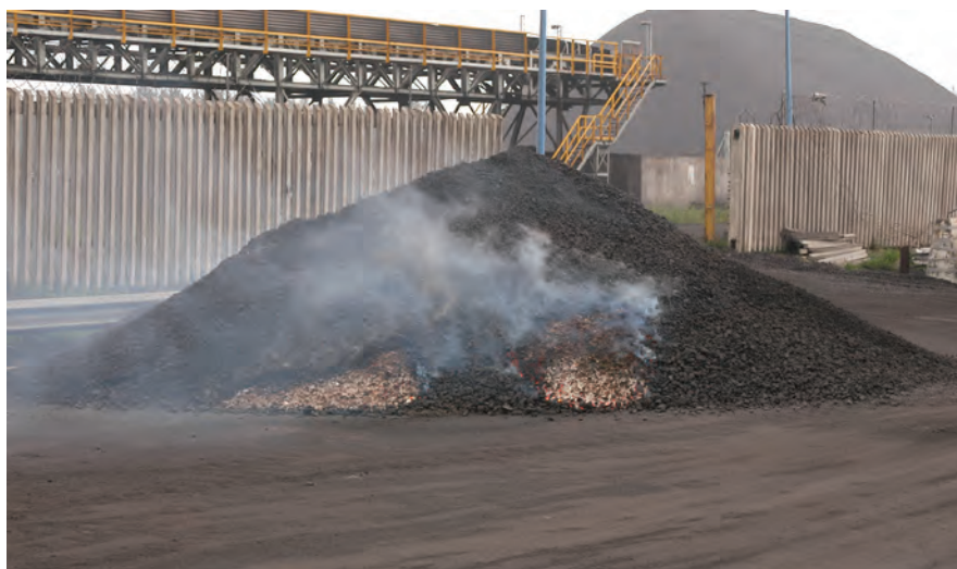
Fig. 36. Coal on fire in a pile on the quay having been removed from the ship's hold
