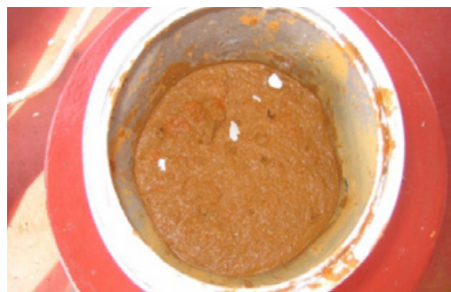
Figure 4: After - on this occasion, the test indicates a higher risk of liquefaction.
