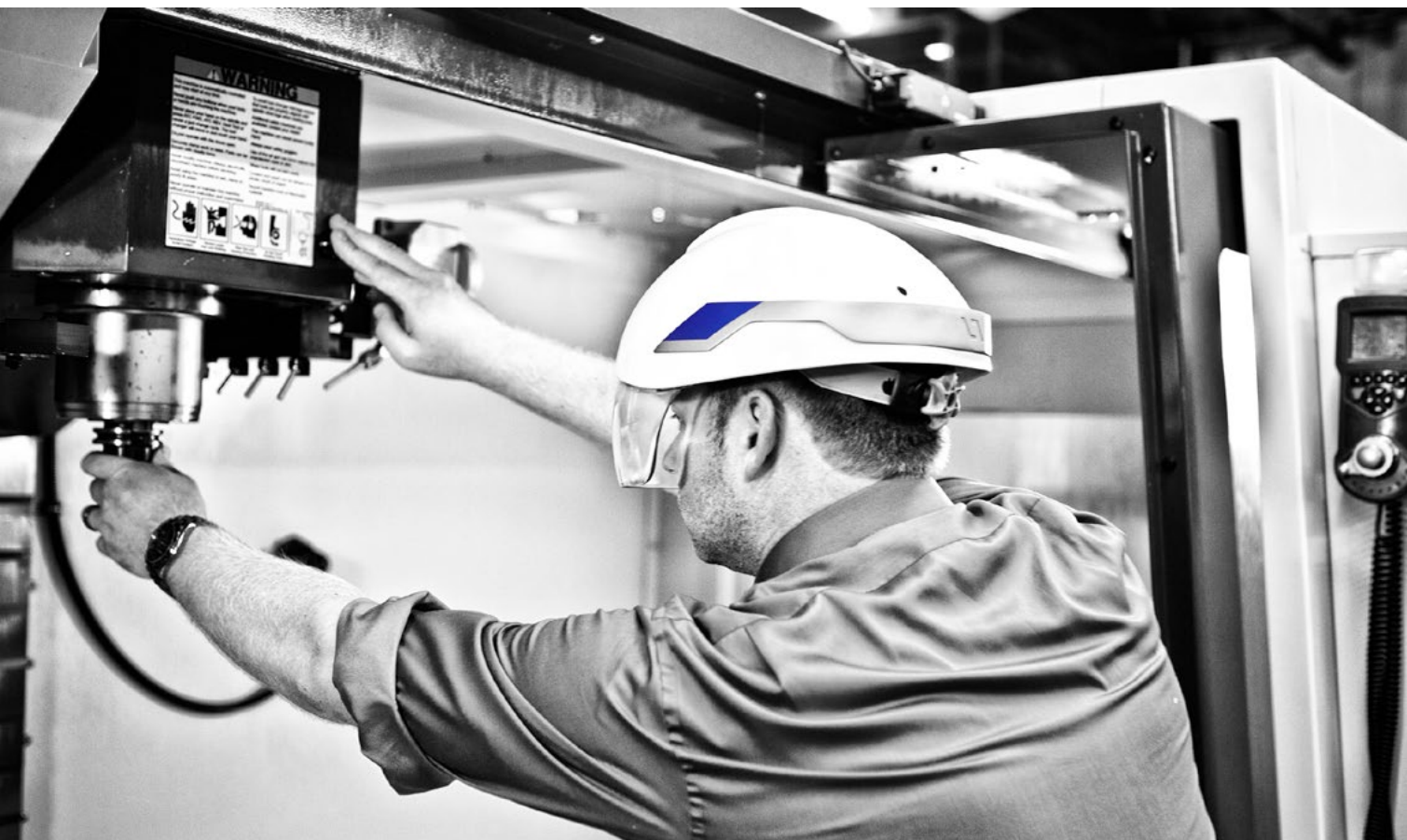
Figure 17. DAQRI's smart helmet contains an integrated display, camera, and sensors. Source: http://daqri.com/
