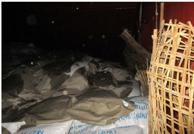
Wet Kraft paper and bamboo dunnage
